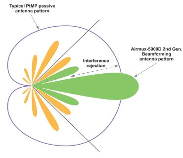
Airmux-5000D 5 GHz beamforming antenna pattern vs. a typical PtMP antenna
