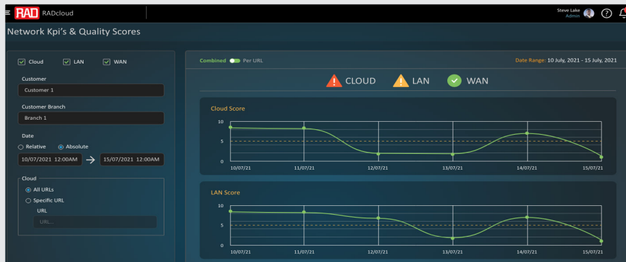
RADinsight high level view: Highlighting problem areas per a specific business site
